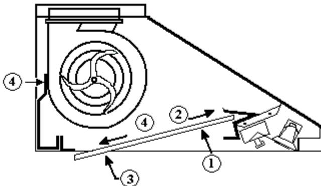
TO REPLACE FILTER PUSH FRONT OF FILTER UP (1)
