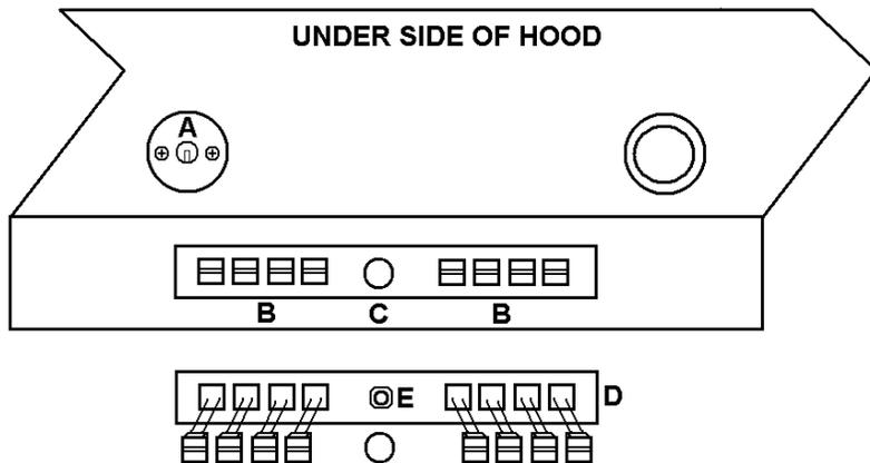
1. Turn Arrow CLOCKWISE to INCREASE voltage to 58VAC on low speed setting.
