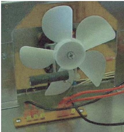
Cap the disconnected wires with the appropriate terminals. Use wire tie to insure wires do not get into the fan blades.
