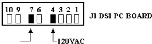
If power is present, check power between 4 and 7. The module will lock out if a call for bake and broil exists simultaneously.
