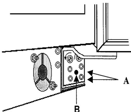
1. To raise the fresh food door, loosen the (4) bolts (A) on the lower hinge mounting plate.
