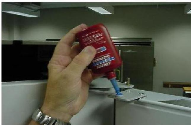
2. Add Loctite (non-hardening) to top of screw.
