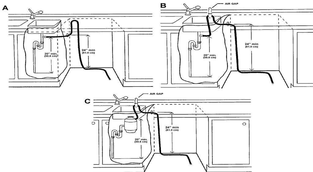
**CAUTION:** Failure to provide either the proper drain connection height (24" [61.0 cm] above floor level) or a 24" (61.0 cm) high loop will result in improper draining of the dishwasher, which will cause damage to the dishwasher.
