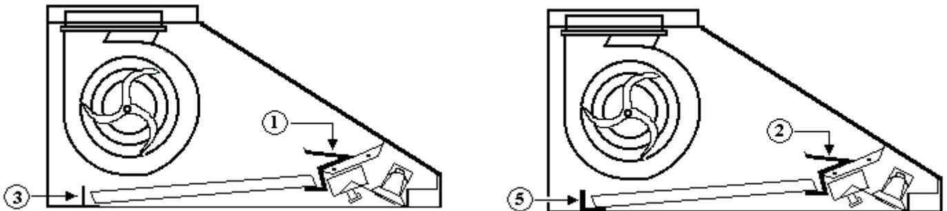
1. REMOVE EXISTING WIRE CHANNEL BRACKET
