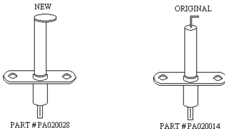
The new igniter is shipped as a kit (G5007447) including six PA020028 igniters. The G5007447 igniter kit will automatically replace PA020014 and PA020028 when ordered from your parts distributor.
