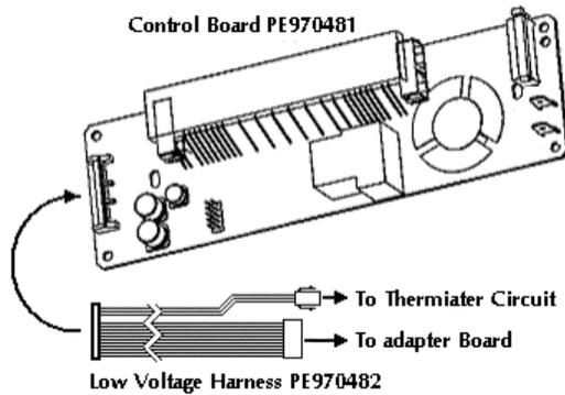
Kit consists of: **Control board PE970481** and **Low voltage Harness PE970482**
