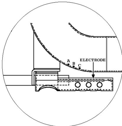
THE IGNITOR ELECTRODE MUST BE IN THE TIPS OF THE INNER BLUE CONE AT PORTS "A" "B" & "C"
