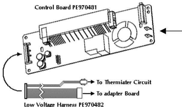
New Low Voltage Board – with light terminal and low voltage harness.
