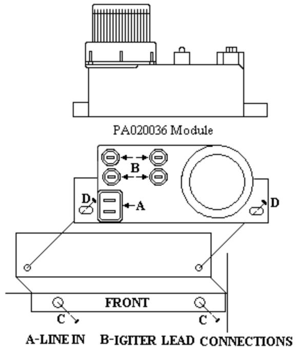
6. For easy access to the Spark module and bracket, remove the drip tray.
