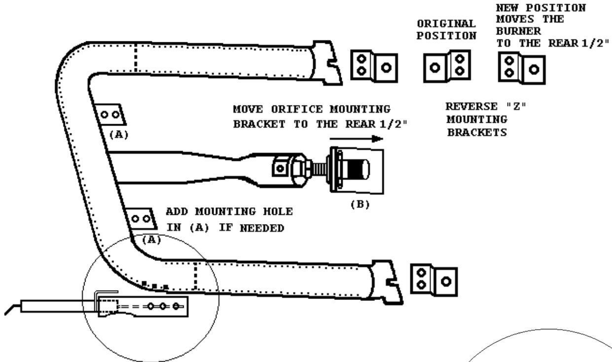
**THE IGNITOR ELECTRODE MUST BE IN THE TIPS OF THE INNER BLUE CONE AT PORTS "A", "B" & "C".**
