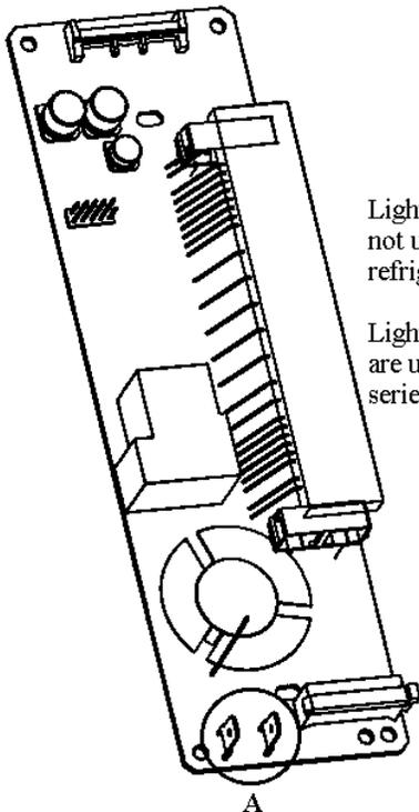
Light Relay Terminals not used on "F" series refrigerators.
