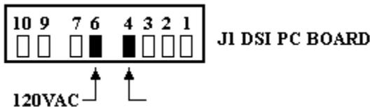
If power is not present, check wiring and/or Thermostat.
