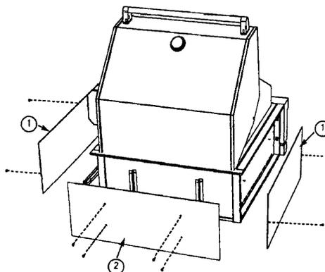
1. To remove the side heat shields (Labeled #1), remove the two (2) screws - one in front and one in back.
