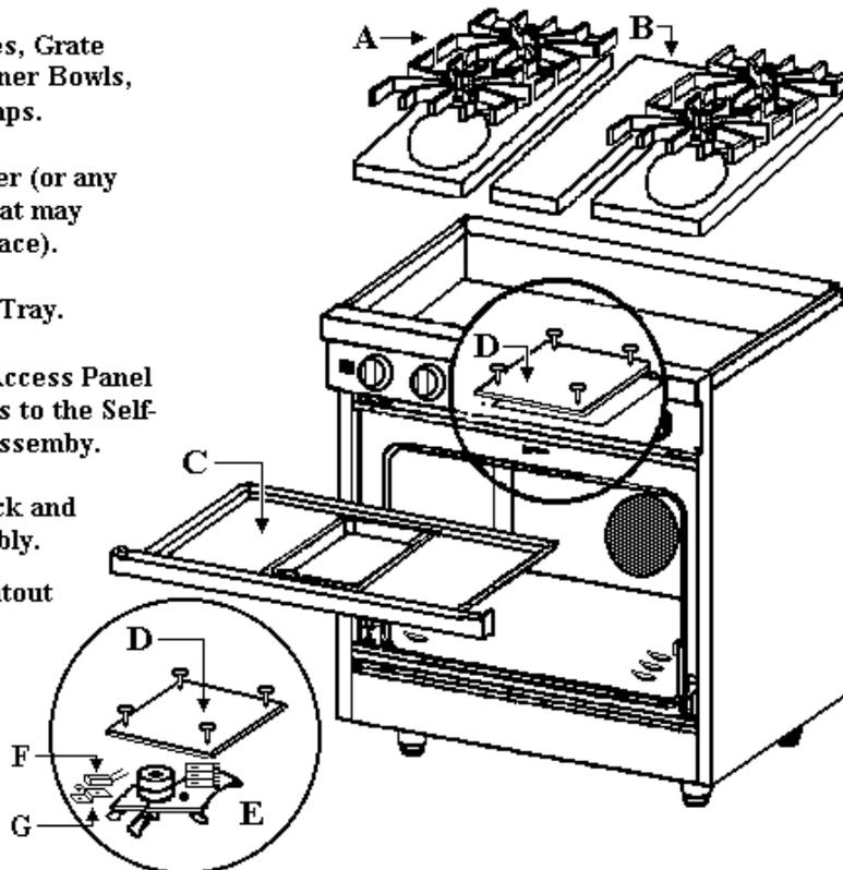
Remove the High Limit Cutout and mount the "Z" bracket in the existing hole. Mount the High Limit Cutout on the "Z" bracket and reverse the disassembly process.
